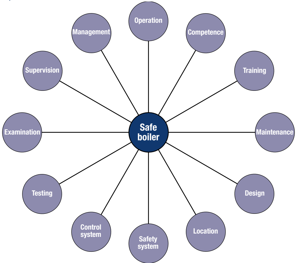
Figure 3 What can affect safe boiler operation?
